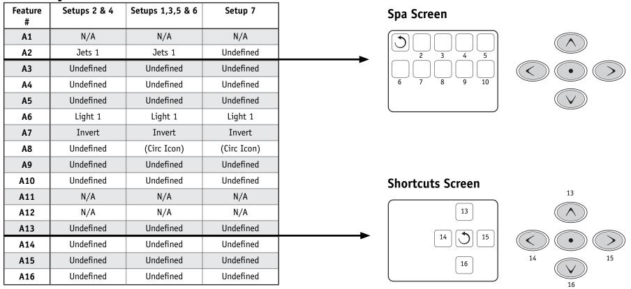
A Circ Icon will appear when a Circ Pump is configured.
