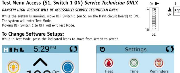
The example screens shown here are from the spaTouch 1 Icon-Driven Panel, but the screens on the spaTouch 2 Panel are similar. The main difference is that the spaTouch 2 display is wider.
