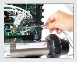
Place the Wi-Fi cable and Control Panel cable inside the wire holder.
