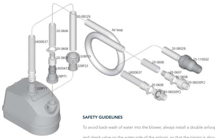
To avoid back-wash of water into the blower, always install a double airloop and check valve on the water side of the airloop, so that the piping is above water level twice. The blower is not to be mounted directly on the floor for safety reasons.
