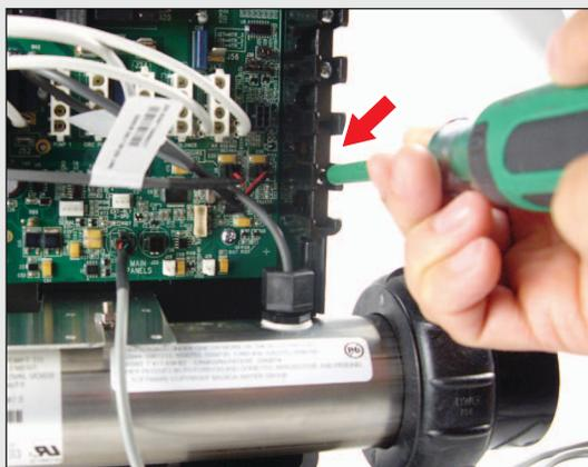
– Remove 1 screw to open the cable holder.
